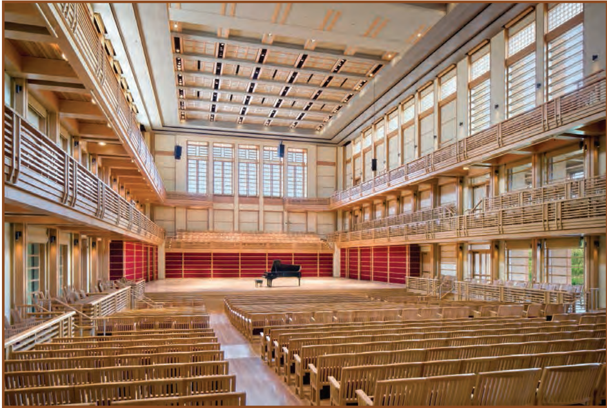
Fabricated by Theatre Solutions from European steamed beech wood, each seat features an open back and a burgundy cushion.
